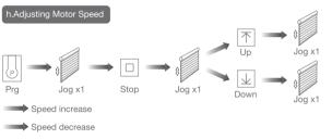
Note: If motor doesn't jog, the max/min speed has already been reached. There are 3 speeds adjustable.
