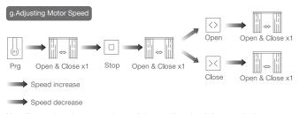
Note: If motor doesn't response, the max/min speed has already been reached. There are 3 speeds adjustable.
